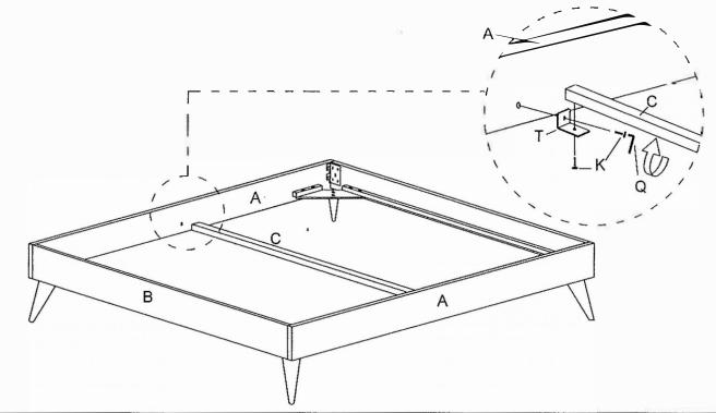
6 Insert JCBC M6 X 70mm (L) into the Center Support (C) by Allen Key M4 (Q), into the Support Leg (D), and turn the Adjuster M6 (S) into the bottom of the Support Leg (D)
