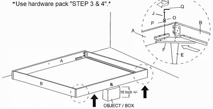
4 Level up the Headboard Panel (A) by putting on object/box to fix the Bed Leg (E) with the Bed Leg Support (F). Insert JCBC M6 X 50mm (J) Flat Washer M6 (P) Spring Washer M6 (O) to Headboard panel (A) connection Bed Leg Panel by Allen Key M4 (Q).
