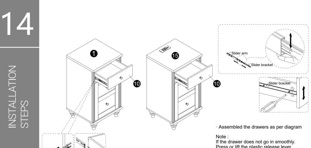
Press or lift the plastic release lever. Pull out the slider bracket from the slider arm.
