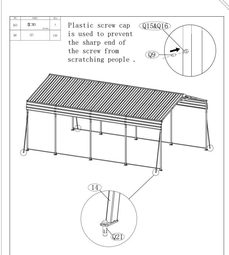
1. It is necessary to use ground nails and expansion screws, whether installed on stable ground, to avoid the collapse of the car shed to the inside or nearby personnel causing devastating injuries and property losses.
