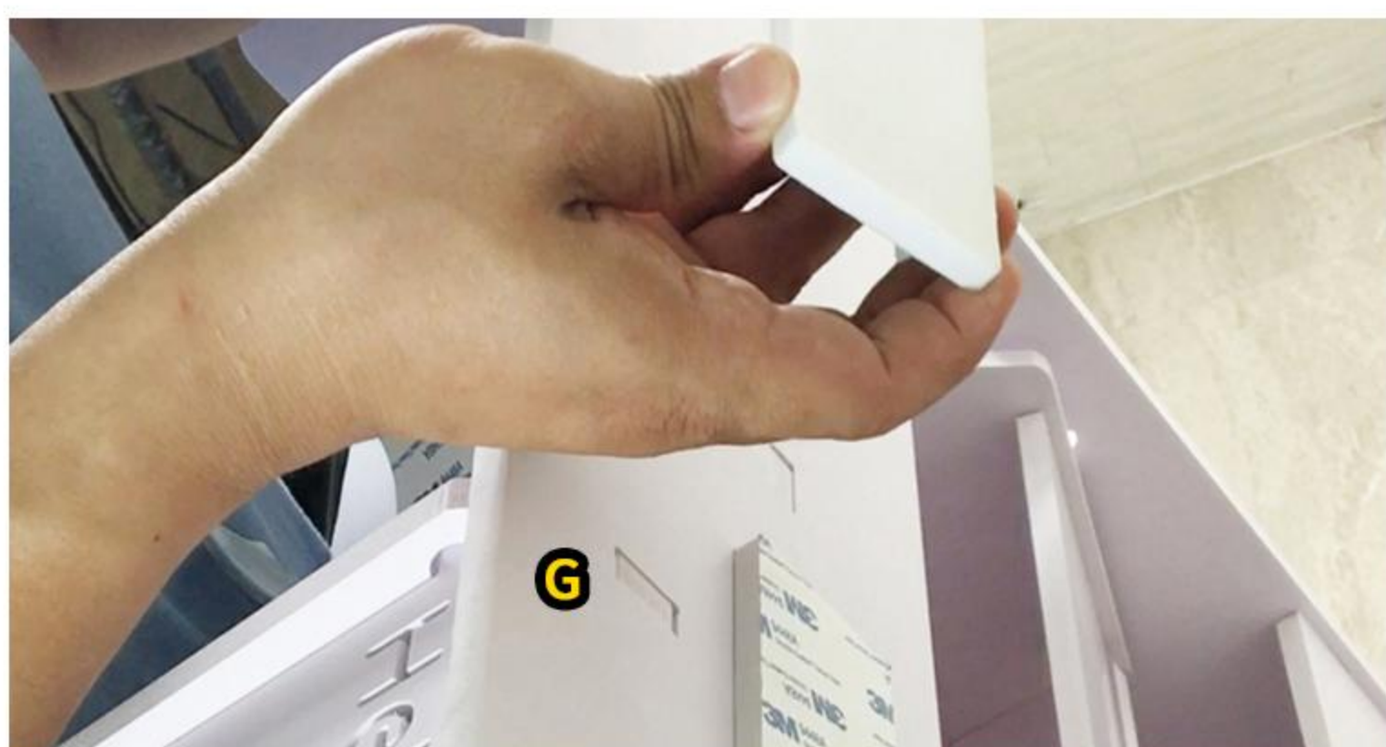
STICK ANTI-COLLISION FOAM ADHESIVE ON THE BACK
