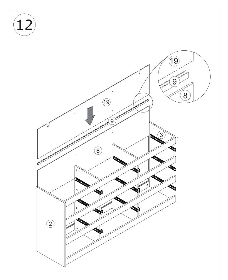
Connect part 19 and part 8 with part 9 and insert into the available slots of part 2, 3 and 7 as shown.
