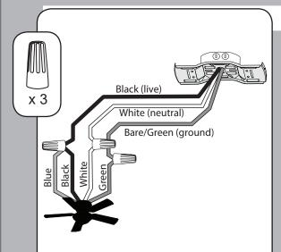
**Note:** If there is a second hot supply wire coming from the outlet box, connect it to the blue (light power) fan wire for separate light and fan control.
