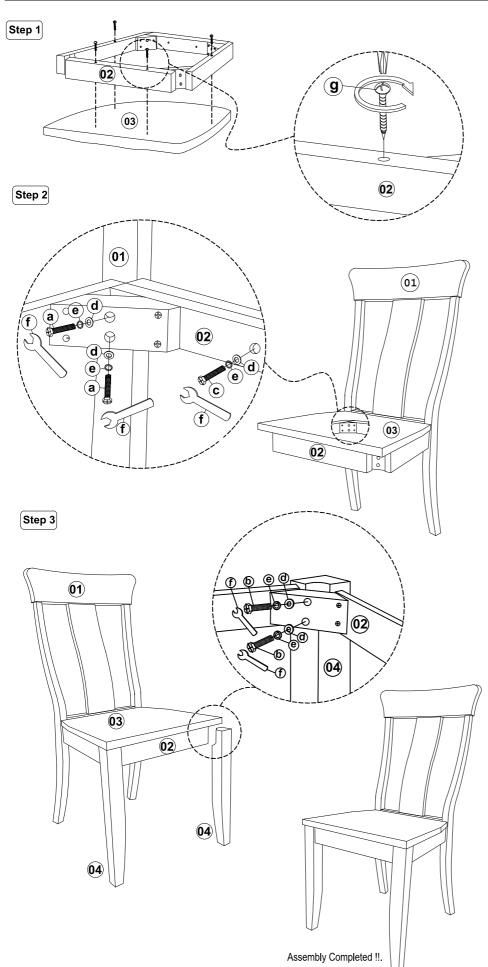
List of Part For 1 Set Code Figure Part Qty. Back Frame (01) 1 Seat Frame 1 (02) (03) 1 Seat Board Front Leg 2 (04)
