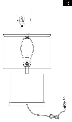
Insert the bulb(G) into the socket(C).
