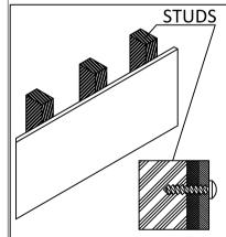
STUDS: Secure to wall with #10 x 3" screws at stud
