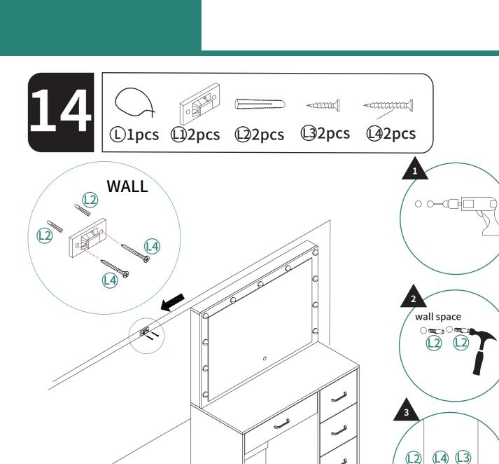
After the cabinet assembly, please install the wall fixing device on the back of the cabinet to avoid accidents.
