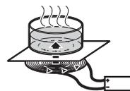
Since the heat required for cooking is generated directly in the base of the pan, the Cooking Zone itself warms up only slightly. The cooktop becomes hot from the heat from the base of the pan.
