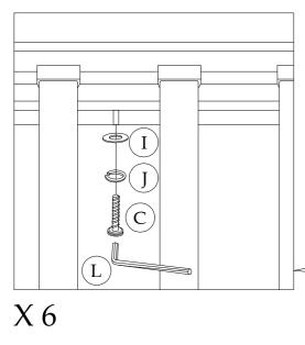
Check that the frame is central by adjusting the alignment of the frame and brackets before fully tightening all bolts. The metal frame should not contact the faux leather at any point.
