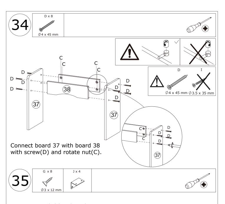
Fix corner code(J) to board 38 with screw(G) as shown.
