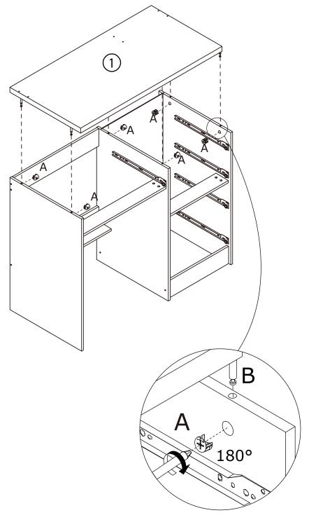
Cover board 1 into the component and turn cam locks(A) clockwise to tighten as shown.
