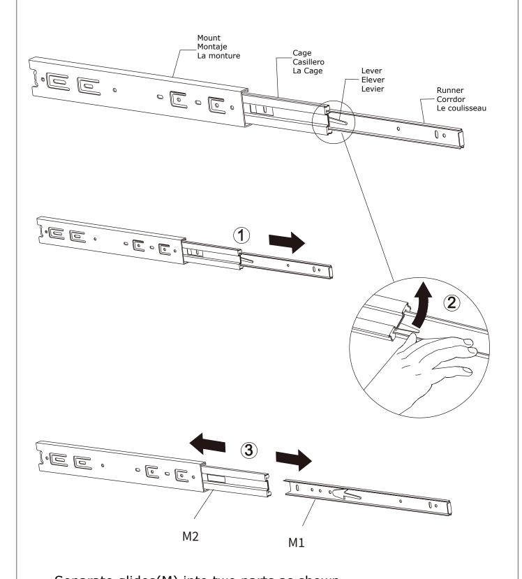
Separate glides(M) into two parts as shown.
