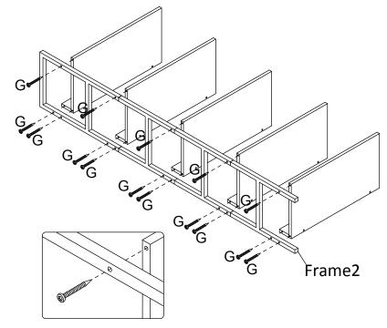
**Step 4**Attached one frame to the right side of the five panels using (G) hardware. Be careful not to overtighten to avoid stripping of the screws.
