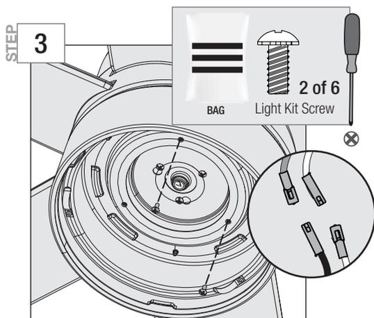
Partially install two of the light kit screws found in the bag. It does not matter which two screw holes you choose. Connect the single-pin connectors from the LED assembly to the connectors from the fan. Connect the white wires together. Connect the blue and black wires together.
