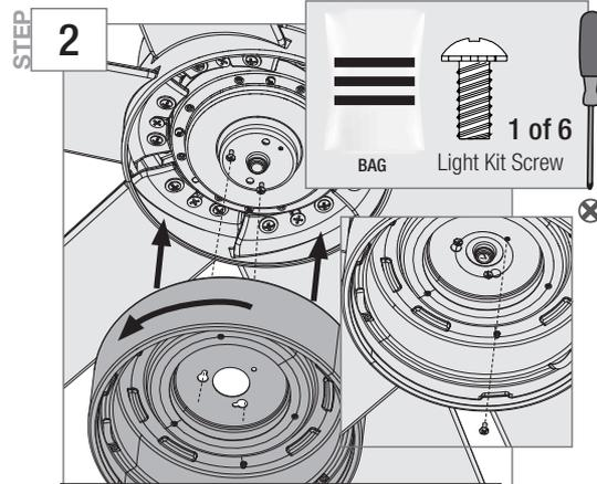
Align the keyhole slots in the top of the light kit assembly with the partially installed assembly screws. Wrap the keyhole slots around the screws and twist counterclockwise. Install the third light kit screw. Tighten all screws securely.
