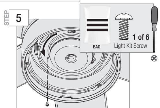
Turn the light kit counterclockwise until the light kit screws are firmly situated in the narrow end of the keyhole slots. Install the third screw and tighten all three screws securely.
