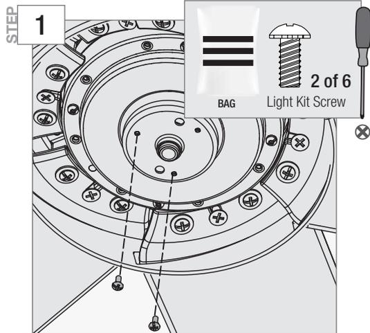
Partially install two light kit screws, found in the bag, halfway into the motor housing as shown. It does not matter which two screw holes you choose.
