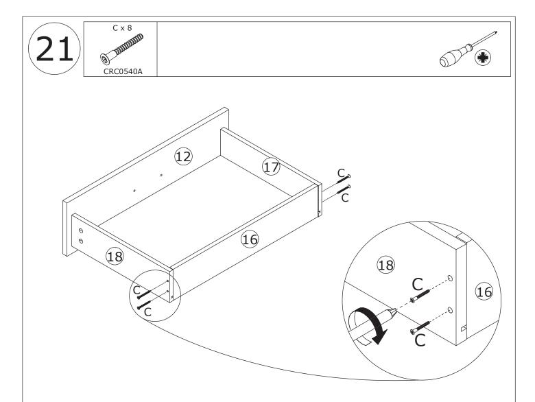
Fix board 16 to board 17 and 18 with screw(C) as shown.
