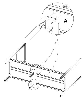
Installation to the cabinet floor after installing fittings 6 and 7 in place
