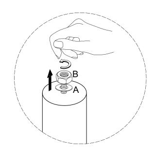
Loosen and remove nut (B) and washer (A) from pole (2).
