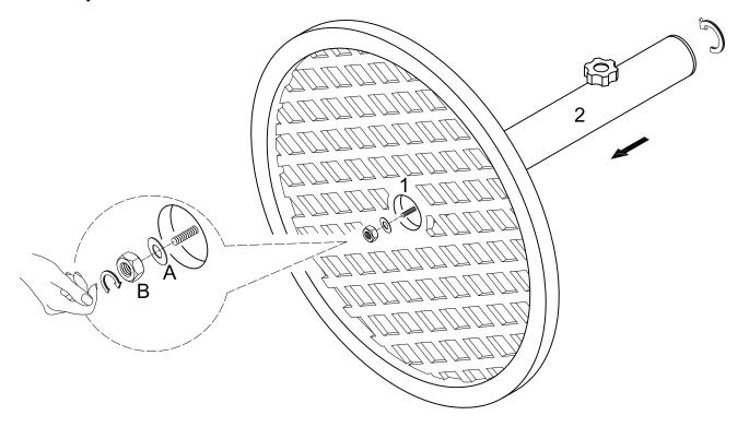
Insert pole (2) into stand bass (1). Secure pole (2) using nut (B) and washer (A). Tighten nut (B) firmly.
