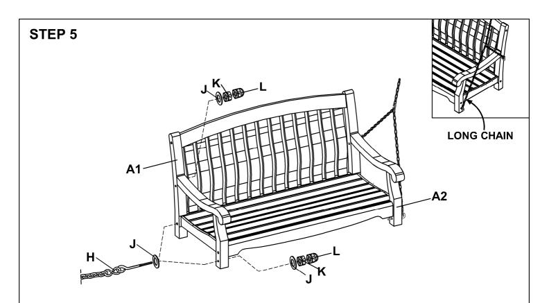
Secure the hanger bolts with chain (H) into predrilled holes of the right side frame (A1) using washers (J), nuts (K), and head nuts (L) as shown. (The hanger bolts with <u>long chain</u> must be install in front). Repeat the same procedure to install the hanger bolts (H) into the left side frame (A2). make sure all parts are correctly connected and tighten all nuts completely using wrench.
