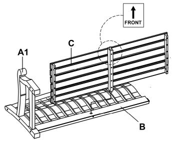
Install on level ground. Attach the right side frame (A1) into Next, attach the seat (C) into predrilled holes of back back support (D). Secure with 2" bolts (E). Do not tighten the bolts yet.
