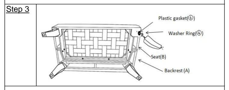
Install the Legs(C) onto the Seat(B) and Backrest(A) by putting Washer Rings(④) and Plastic gasket(⑥)(optional but improve security and tightness) onto the theaded stem.
