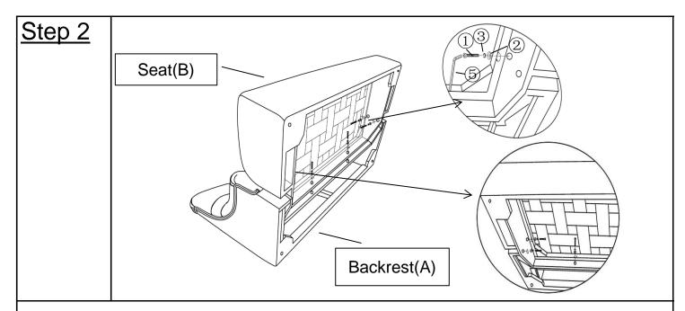
Place the Backrest(A) faceup on the floor, then slide the Seat(B) into the housing.
