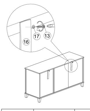
4. Add safety strap (16), washer (17) using 3.5x15mm screw (13) to back of cabinet.
