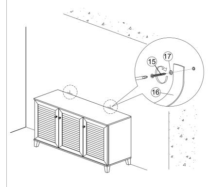
5. Finally, attach safety strap (16) and washer (17) using 4x30mm screw (15) to the wall.
