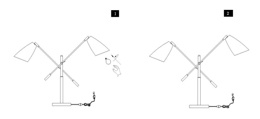
Step 1 Insert the bulb(B) into the socket.
