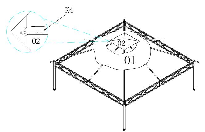
Put Small Canopy(O2) on small roof frame, fix four corners to Short Extension Tube(K4) and adjust tube to suitable length.
