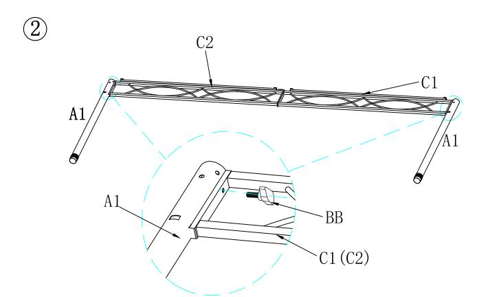
Connect Top Leg Post(A1) to assembled Corss Beam 1/2(C1/C2),locking by Bolt BB.
