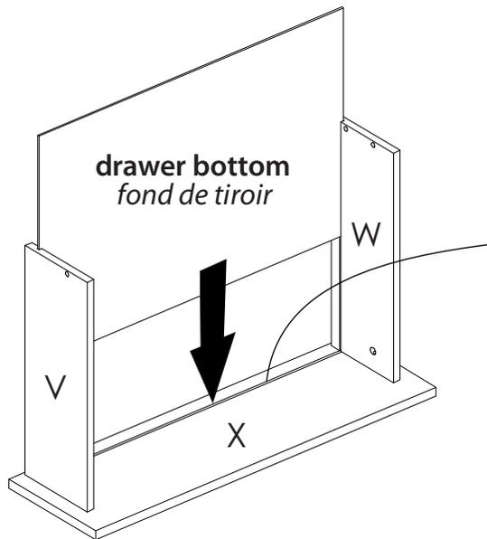
**Drawer bottom must enter into the groove located on panel X**
