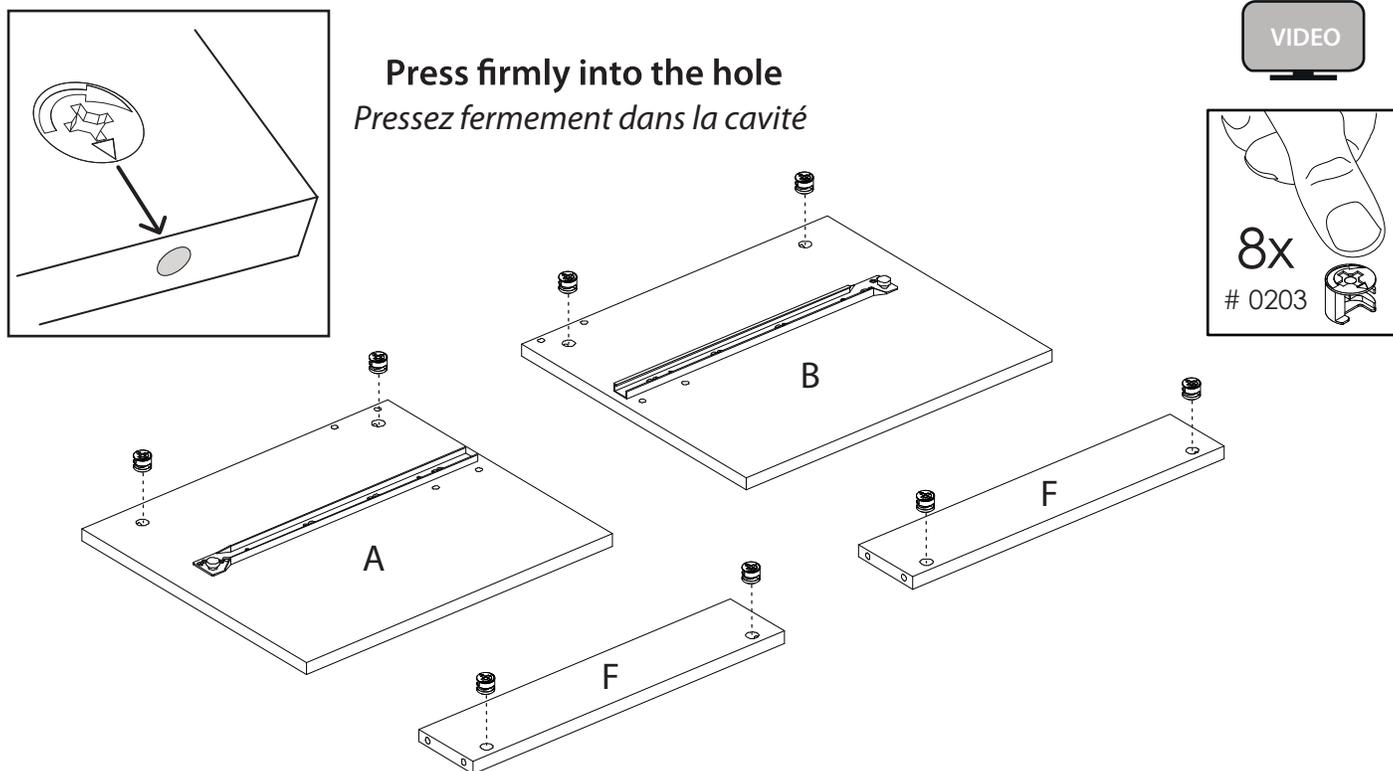
**3** Install 8 push bolts # 2200 into the panels A, B and C
