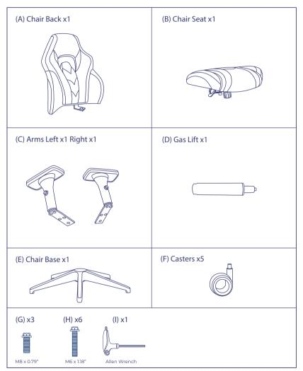
03 How to Assemble Cobra
