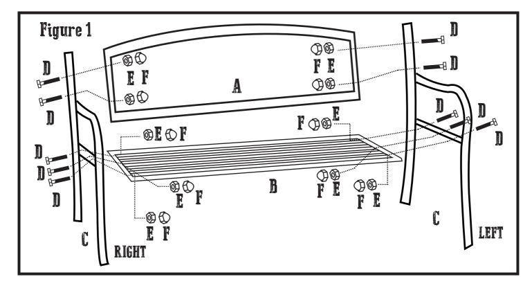
1. (SEE FIGURE 1) Take the Seat Panel (B) and align the holes to the holes of the Arm Frame (C) and secure by inserting Botts (D) through the Arm Frame then Seat Panel. Secure the Botts (D) with the Hex Nuts (E) on the inside of the Seat Panel. Repeat for the other the Arm Frame (C).
