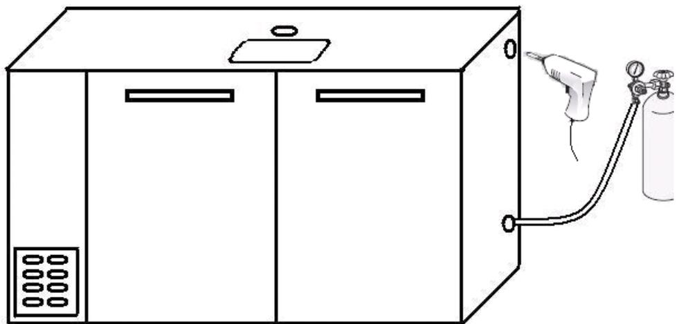
1. Drill and bore a hole through the wall in either of the places where the foam insulation is exposed.
