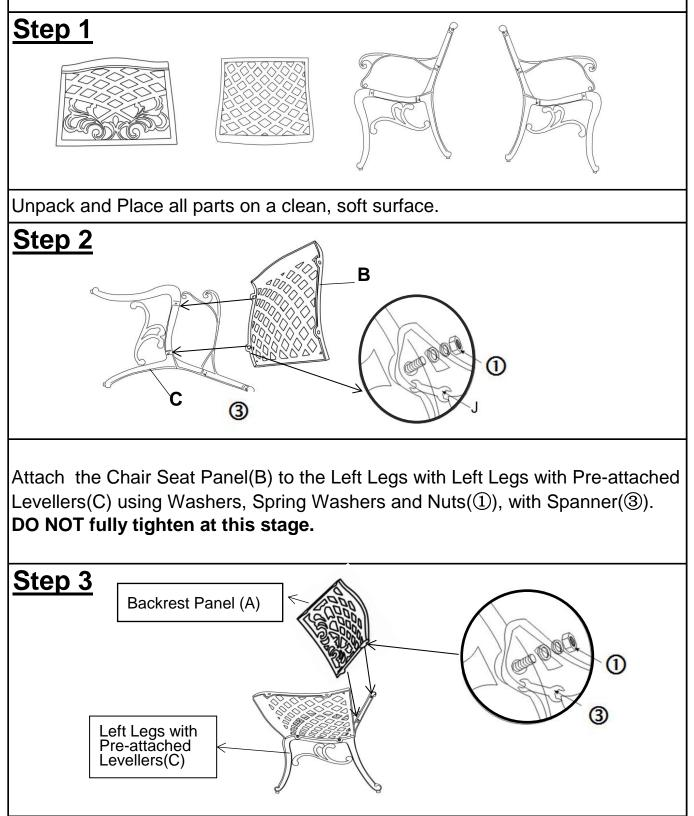
Then attach the Backrest Panel(A) to the top end of the Left Legs with Preattached Levellers(C)using Washers, Spring Washers and Nuts((1)) with Spanner((3)).
