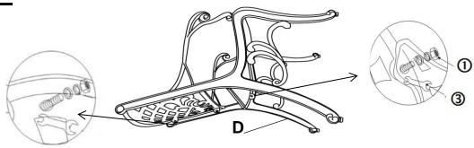
Repeat the same assembly process for the Right Legs with Arm and Preattached Bolts for Seat Panel and Leveller(D) **DO NOT fully tighten at this stage.**
