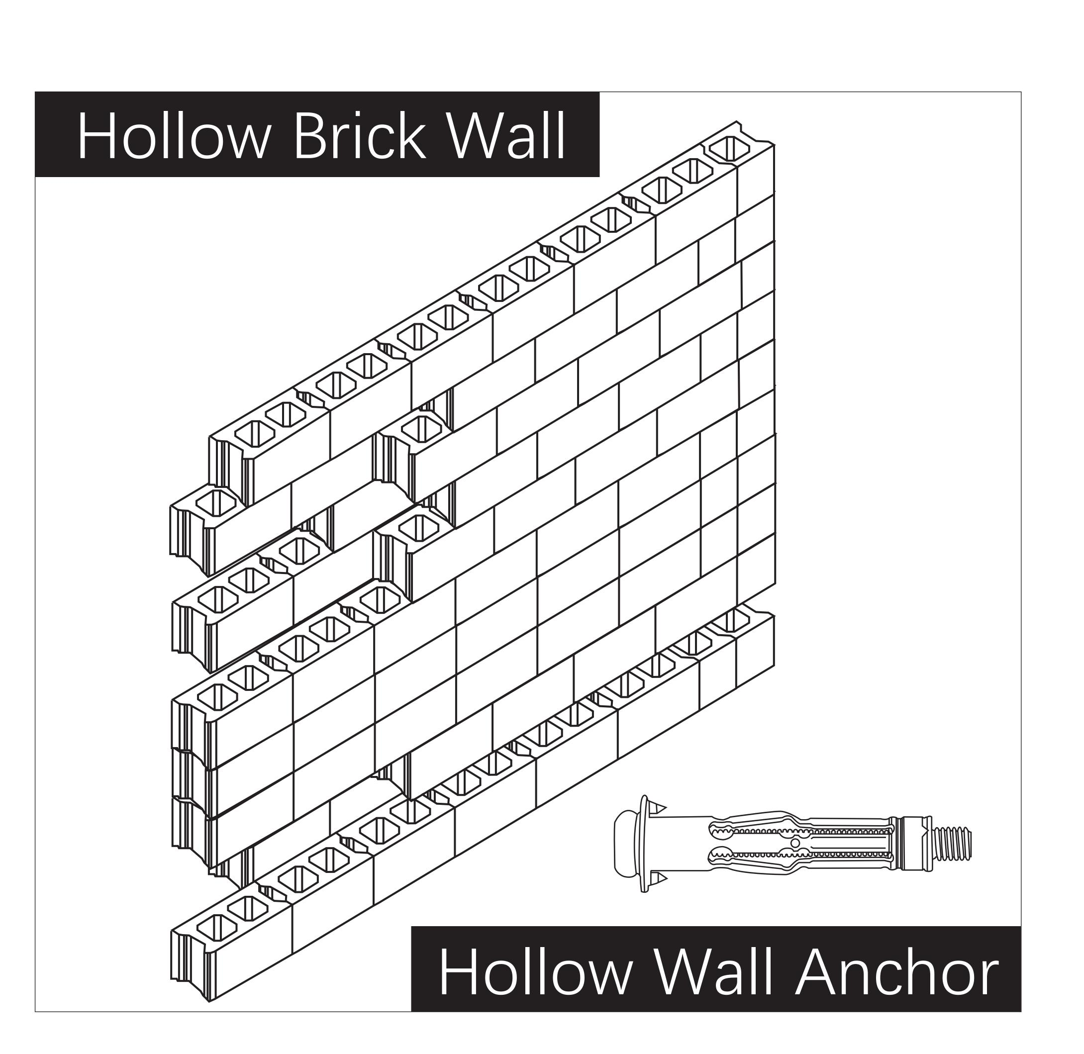
Please use hollow wall anchors (not included) for installation on hollow brick wall.
