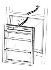
6. Insert and secure the cabinet; hardwire the power cord according to local electrical codes. Connect the load (black) wire of the Light cable (white) to wall switch if used. Connect the load wire of the Outlet cable (black) to hot wire.
