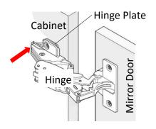
1. Unplug the cable from the Mirror Door to electrical enclosure. Remove the Mirror Door by pulling on the tab behind the Hinge to detach the hinge from the Hinge Plate. Remove the TOP hinge plate.
