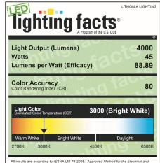
All results are according to IESNA LM-79-2008: Approved Method for the Electrical and Photometric Testing of Solid-State Lighting. The U.S. Department of Energy (DOE) verifies product test data and results.
