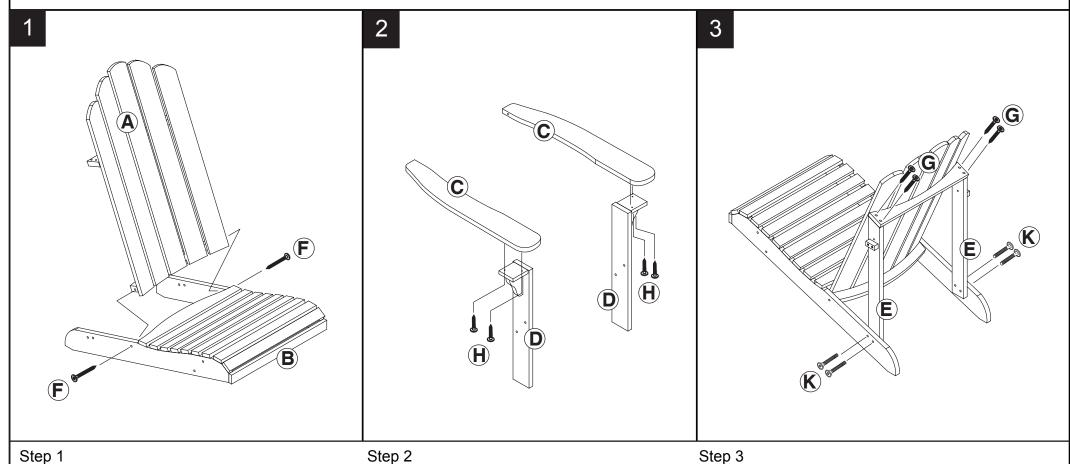
Attach back frame (A) to seat frame (B), by using Screw (F), tighten with allen key(L)
