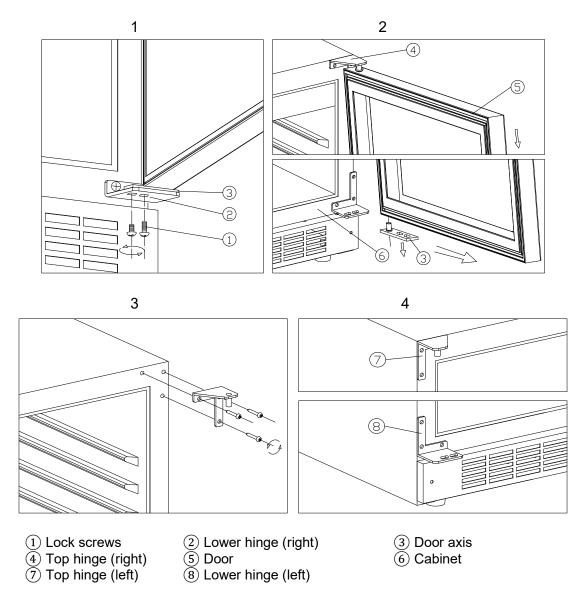
Unscrew the Lock screws (1) (Fig. 1)
