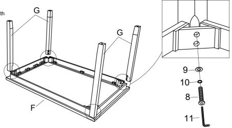
STEP 3: To level the table, stand the table up on a flat surface and tighten all the bolts by using Allen Key (11).
