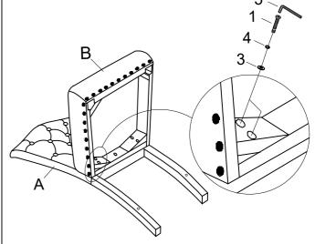
STEP 3: Assemble the front legs (C&D) with the Cushion Seat (B) by using Allen Key (5) with hardware 1, 2, and 4.
