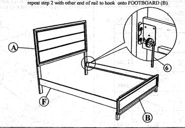
STEP 3: Tighten the 4 Corner with Allen Key (6). Fix the Bed Slat Support Leg (E) to Bed Slat (D) Install the bed slat (D) to side rail (F) and tighten with Csk Screw (1) as per diagram shown. (NOTE: THE SETUP MUST DONE AT THE DECIDED LOCATION FOR THE BED TO OBTAIN PERFECT STABILITY)
