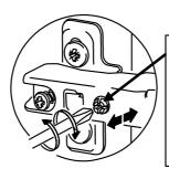
**Horizontal Door Adjustment: Rotate Screw clock wise or anti** clockwise. This will produce an even gap between doors and frame.
