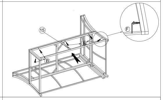
STEP 4: Connect The Part from Step 3 and Corner Front Frame (15), tighten Allen Bolt (B), Flat Washer (E) with Allen Key (F).
