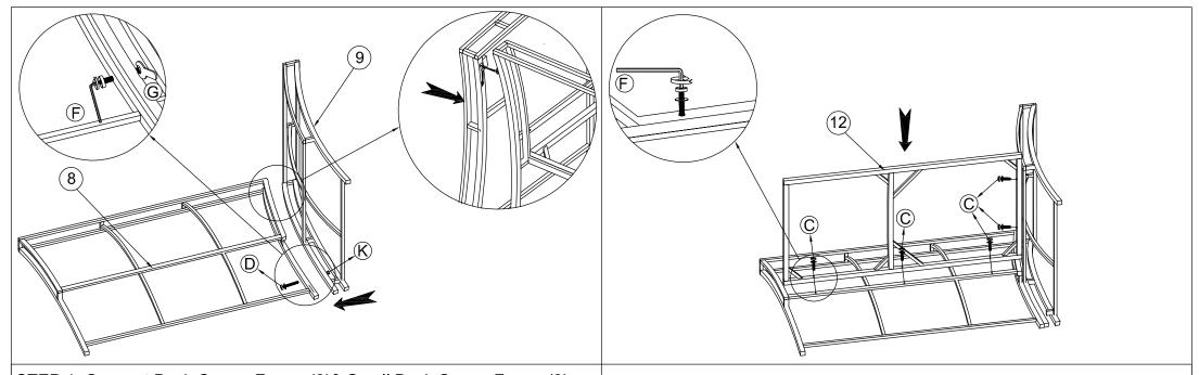
STEP 1: Connect Back Corner Frame (8)& Small Back Corner Frame (9), tighten Allen Bolt (D), Flat Washer (E)& Eru (K) with Allen Key (F) & Key (G).
