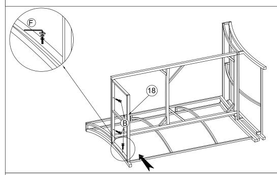
STEP 3: Connect The Part from Step 2 and Corner Side Frame (18), tighten Allen Bolt (B), Flat Washer (E) with Allen Key (F).
