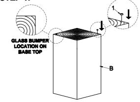
BUMPERS SHOULD BE APPLIED TO BOTH PEDESTALS TO PREVENT GLASS FROM MOVING.
