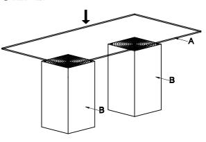
POSITION PEDESTALS UNDER GLASS TOP TO PROVIDE MAXIMUM SUPPORT DURING USE
