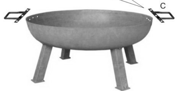
STEP2 FIX THE HANDLES INTO THE FIRE BOWL WITH BOLTS, NUTS & GASKETS
