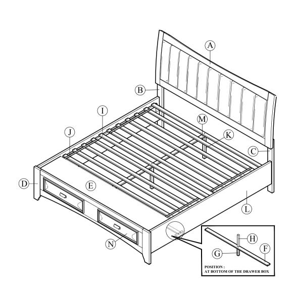
STEP 1.1: Align and fasten Headboard Leg (B) & (C) to Headboard Panel (A) using JCBC M6 x 30mm (1), Spring Washer  $\emptyset_4^{1}$ "(2) and Flat Washer  $\emptyset_4^{1}$ " x 13mm (3) and tighten with L Key M4 (7). \*\*Please note the marking on the leg and headboard\*\* "R" Marking behind the
