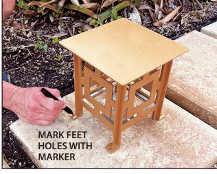
Mark feet holes with marker, don't forget to mark the hole for the low voltage wire to connect to the Lamp.
