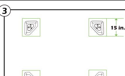
Or you can make a concrete footing for gazebo,  $15 \times 15 \times 15$  inches is recommended use expansion bolts to mount the pergola like (2) shows.
