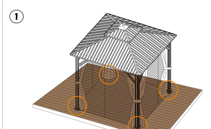
If the deck is hard wood and the depth of it is over 3 inch, you can use 5/16 in. ×4 in. Structural Wood Screw to mount the gazebo.
