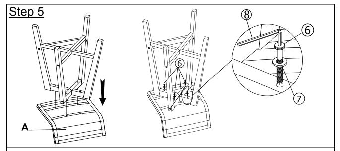
Place the Seat Panel (A) onto the surface as shown above Insert assembled frame on step 3 into Seat Panel(A) using Bolts(6) and Washers (7) with Allen Key(8) as pictured above.
