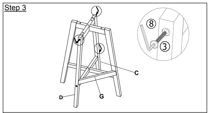
Attach Second Leg (C), Third Leg (D), Third Cross Bar (G) to the assemble on step 2 using Bolt (3) and Allen Key(8) as shown above.
