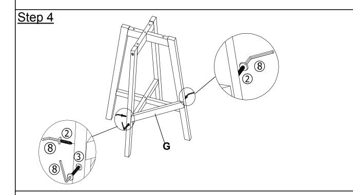
Secure Third Cross Bar (G) to the assemble on step 3 by using Screw (2), (3) with Allen Key(8) as shown in picture above.
