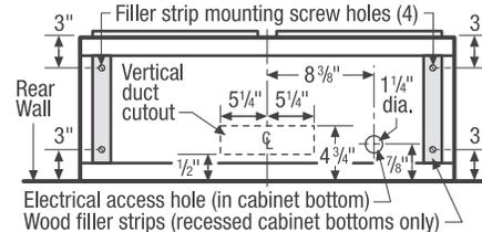
Electrical access hole (in cabinet bottom)
