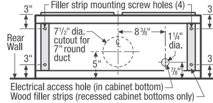
Electrical access hole (in cabinet bottom)
