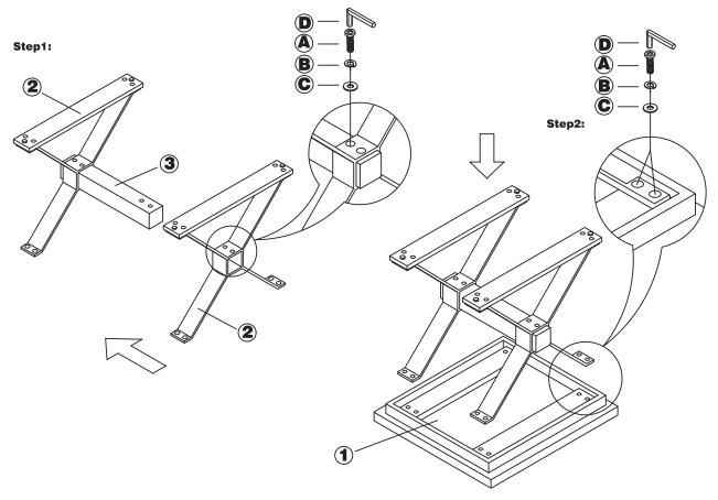
NOTE: DO NOT TIGHTEN ALL THE BOLTS UNTIL THEY ARE INSTALLED IN CORRESPONDING HOLES!
