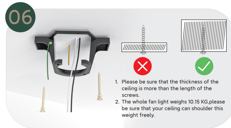
Secure hanger bracket.
