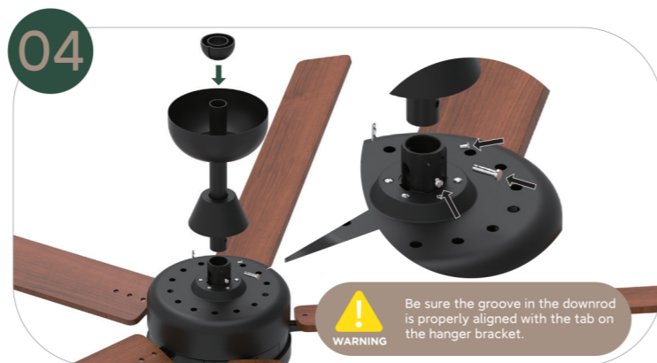
Install the downrod assembly the canopy and the coupling cover in turn.
