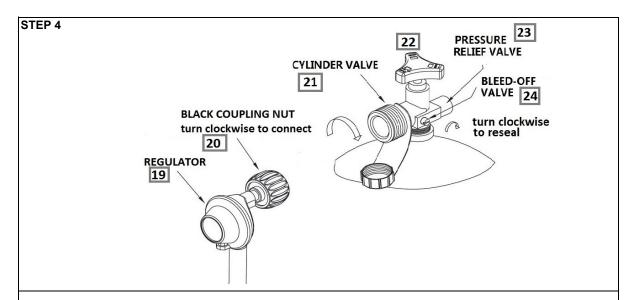
4. Turn the Cylinder Valve (21) on the tank in a clockwise direction to TURN OFF SUPPLY of the LP Gas supply.
