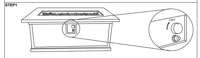
1. Check that the Control Knob (13) for the gas supply system is turned to the "OFF" position before starting any assembly.
