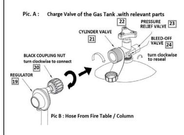
Step 1 : Plug the Black Coupling Nut on the Regulator to the Cylinder Valve.
