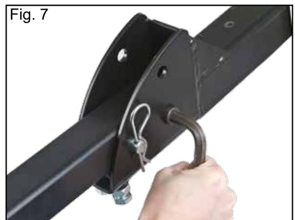
**Step 8.** Adjust the leveler bolt to align the pin holes. The pin with clip (E) should be able to be removed/installed without binding if properly adjusted. Tighten the jam nuts when properly aligned using a 17mm or 11/16" wrench.
