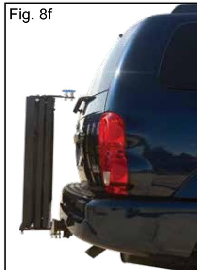
**Step 9.** To unfold the loading ramp, pull the spring pull pin (G) on the carrier basket and lift the ramp up. Next, pull the ramp bracket spring pull pin (F) to allow the ramp to pass. Finally, lay the loading ramp flat on the ground and load wheeled cargo. After the cargo has been loaded, store the ramp in the vertical position. To store in the vertical position, lift the ramp back up and secure using the ramp bracket spring pull pins. Safely secure all cargo with high quality tie downs.
