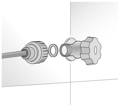
The models provided with Ice Maker require a connection to the domestic water supply system. This can be executed through the 1/4" water line (copper or polyethylene) to the house water supply. The system pressure must be between from 8 psi to 75 psi (between 0.5 bar and 5 bar).
