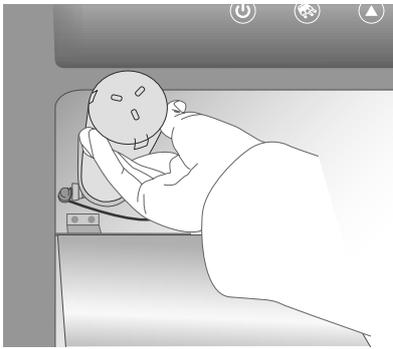
The filter is located inside the refrigerator compartment, above the top glass panel. Prior to changing the filter, switch off the Ice Maker by pressing the IceMaker button. Then enter the Access Menu and set "Manual Clean" function. At the end of the cleaning cycle remove the water from the ice tray and wipe it dry.
