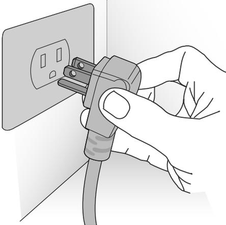
The appliance operates at 115 V AC, 60 Hz and is equipped with a power supply cord with a 3-prong grounded plug, which must be connected to a corresponding 3-prong (15 Amp) grounding-type wall receptacle.
