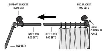
Install this rod (Rod Set 2) by inserting screws through the holes of the brackets. Secure and tighten the rod by turning the screw clockwise.
