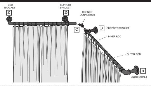
Untighten all the security screws by turning it counterclockwise on support brackets (B, D).
