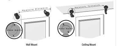
MAKE HOLES ON WALL/CEILING If screws are going directly into wood trim or wall/ceiling studs, drill a 1/8" pilot hole at pencil marks. If screwing into drywall, drill 3/16" (5mm) holes and push or lightly hammer plastic anchors into holes. Then install screws through brackets. Do not tighten screws too much - just snug is best.
