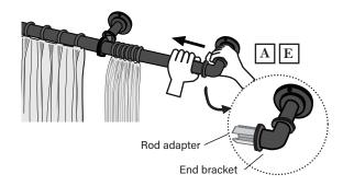
Firmly hold corner connector with one hand and slowly pull the rod out of the corner connector (C) with the other hand. Gently nudge if necessary. Do not twist the rod to avoid misalignment. Rod adapter will stay on the corner connector.
